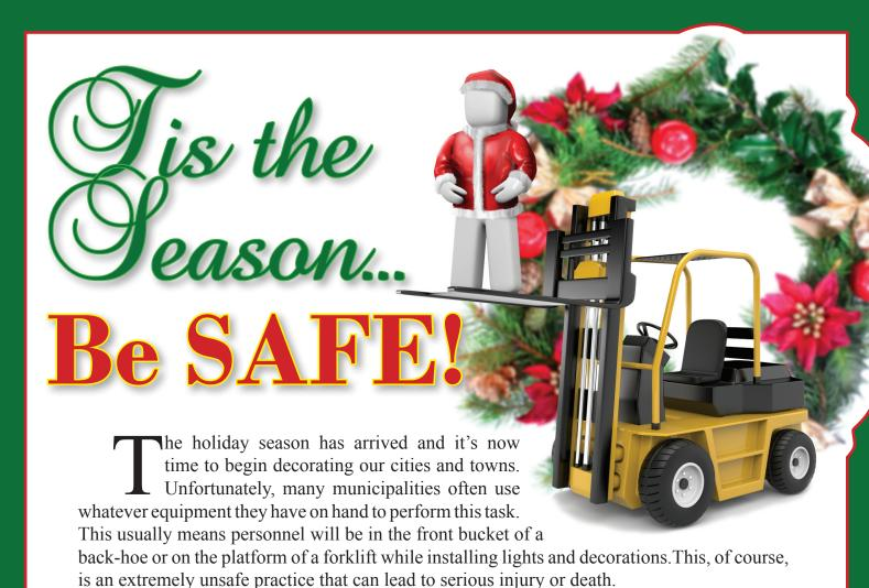
Forklifts and front-end loaders are not designed to lift personnel or to be used as a work platform. OSHA states that forklifts, front-end loaders and "similar pieces of equipment" shall not be used to support scaffold platforms unless specifically designed by the manufacturer for such use. Keep in mind that while OSHA guidelines may not be *required*, OSHA is still a reliable source of information for developing your public entity's best practices.
